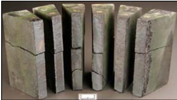
Conventional refractory after rotary slag testing
