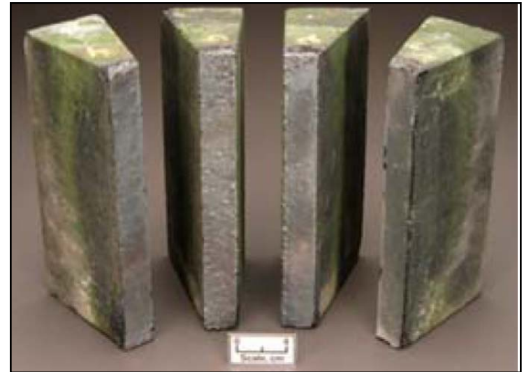
Phosphate modified high-chrome oxide refractory material
